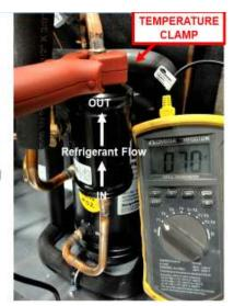
Inlet and Outlet temperature readings are to be taken in both the heating and the cooling modes. Refrigerant temperatures will differ between heating and cooling mode and a restriction may not be seen in one mode or the other, especially if the restriction is caused by moisture in the system. Testing in both modes is critical for an accurate diagnosis.
